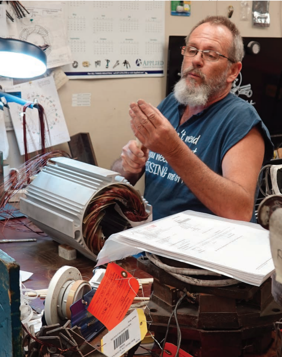
In the servo shop at the St. Bernard facility, Jim Horton winds a servomotor's stator.
